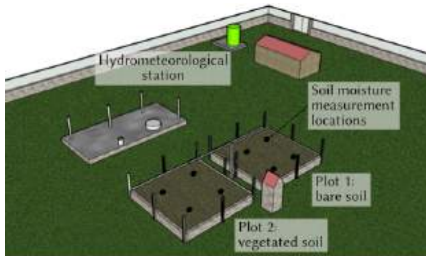
Figure 4.3 - Schematic representation of the field experimental system.
